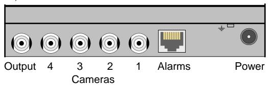
A supplementary earth connection can be made under the screw shown above. Use a small ring terminal crimp.
